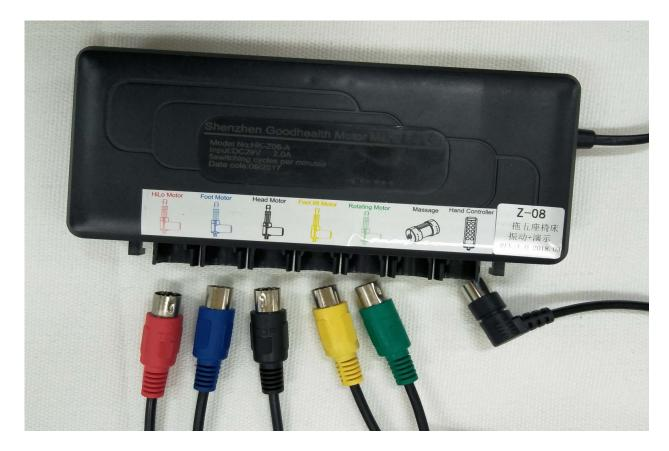
Note: To replace parts and for ease of ordering, all motors are color coded, pictured, and labeled.
